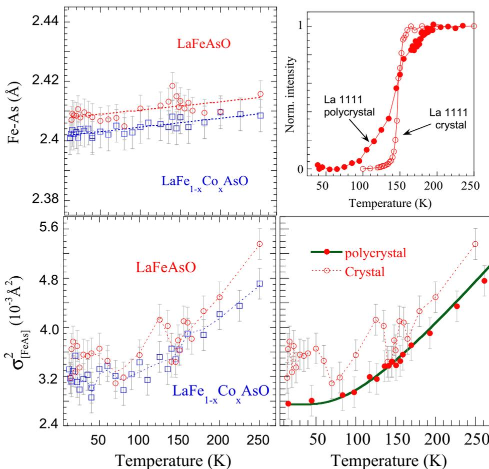
distance and the related MSRDS, describing the correlated Debye-Waller factor ( $\sigma^2$ ), extracted from the above-mentioned single shell modelling of the As K-edge EXAFS data. The Fe–As distance for the Co-doped sample is slightly lower than that for the undoped sample in line with the reduced lattice parameters for the Co-doped [47] sample.
