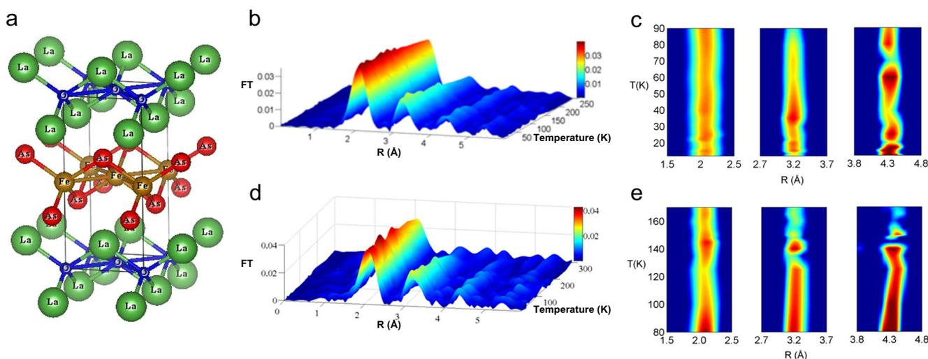
**Fig. 1** Unit cell of  $\text{LaFeAsO}$  (a). Fourier transform (FT) magnitudes of the As K-edge EXAFS oscillations at different temperatures for the  $\text{LaFe}_{1-x}\text{Co}_x\text{AsO}$  ( $x = 0.11$ ) (b, c) and  $\text{LaFeAsO}$  (d, e) single crystals.
